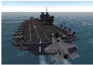
Computer generated image of an F-35B making a rolling vertical landing on a QE class carrier (BAE Systems image)
