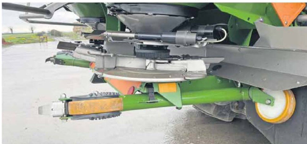
Check that the vanes are in good working order.
