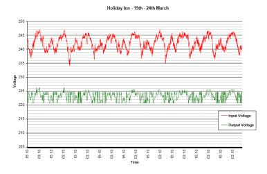
The graph above shows the optimiser provides a stabilised reduced voltage to the hotel, whilst ensuring it remains above 221v, and the integral power factor correction improves the power factor from 0.86 to 0.97.
