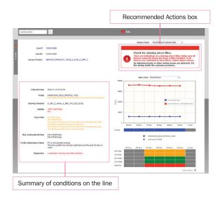
**FIGURE 2.** ClearView graphical user interface snapshot showing the recommended high-level action, detailed guidance for the field technician, and explanations for the conditions on the line.
