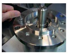
12. Tighten the 4 flange screws to a torque of  $8 \pm 1$  Nm using the tool provided.
