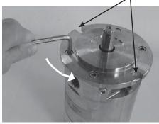
2. Wet the shaft and shaft seal with clean (filtered) soap-water. Gently lever the shaft seal assembly free using 2 screwdrivers.
