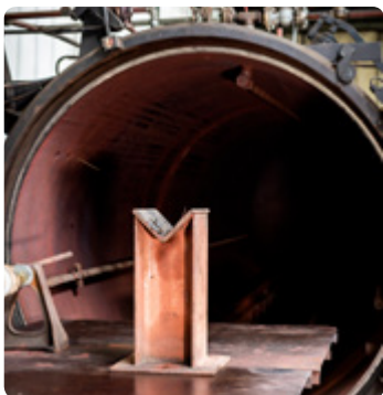
Above: The lining is applied; Below left: Regal's large steam autoclave; Below right: Rubber lined power block sheave.
