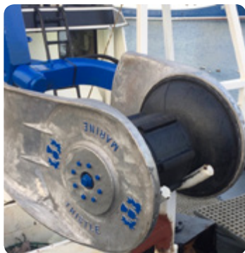
Above: The lining is applied; Below left: Regal's large steam autoclave; Below right: Rubber lined power block sheave.
