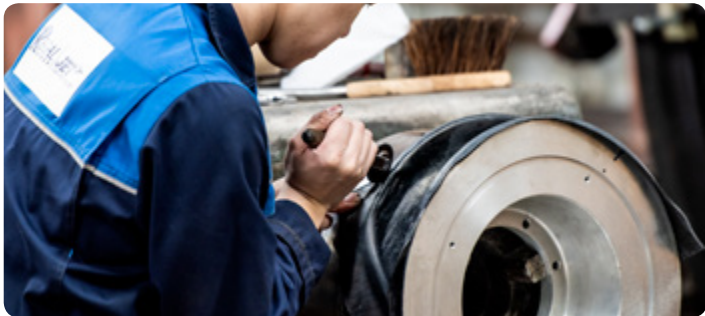
Above: The lining is applied; Below left: Regal's large steam autoclave; Below right: Rubber lined power block sheave.
