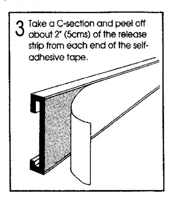
A Make sure the longer lip of the C-section is uppermost and line up its top edge with the top of the glass shelf, lightly pressing down the ends to secure it. Then pull the release strip away completely and press the C-section **firmly** into place. Fit other C-sections in the same way, making sure they butt tightly.
