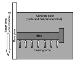
Fig. 3. Bearing force of concrete
