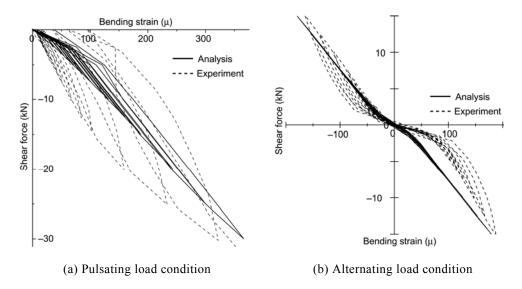
Fig. 9. Shear force-bending strain relations at mid height
