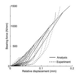
Fig. 6. Bearing force-relative displacement relation
