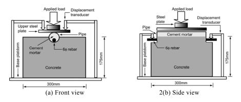
Fig. 2 Bearing test specimen
