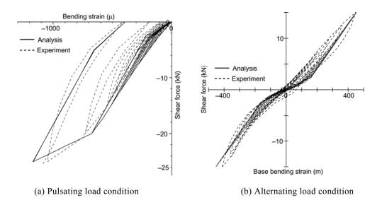
Fig. 8. Shear force-bending strain relations at base
