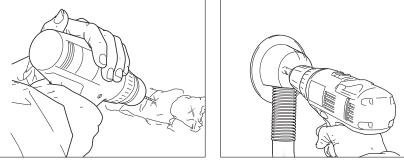
Drill through paste or foam or use a plastic cowl and a Class H vacuum cleaner. A hand drill creates less dust. If you have to use an electric drill, put it on the slowest setting.
