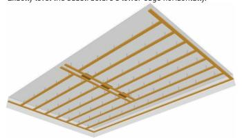
Installation substructure directly to the building structure,
