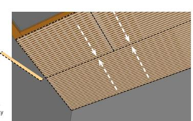
• If special NF type elements are being used, this cut must take place in any case, because otherwise, the gap width at the lateral element joint does not exactly correspond to the gap width in the element surface.
