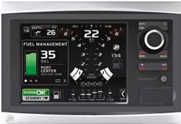
VesselView 7 monitors up to four engines
