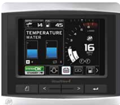
VesselView4 monitors up to two engines
