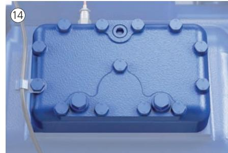
Intermediate adapter for discharge line valve
