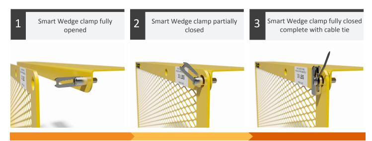
**Please Note:** A cable tie or other device, as shown above, MUST be installed through the Wedge Clamp in the "closed" position to ensure compliance with ANSI B11.19-2010 sec. 7.2.6 and Canadian Regulatory Standards (CSA Z432-16 sec. 6.3.3.2.2) that require a "tool to remove".
