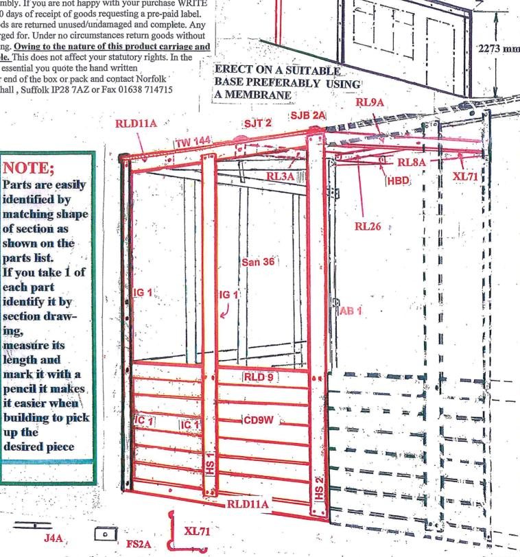
Firstly choose the position for your sunroom. If the wall is rough make up a frame using 3"x1" timber and fix back as shown, sealing the back with mastic and fixing it with rawl
