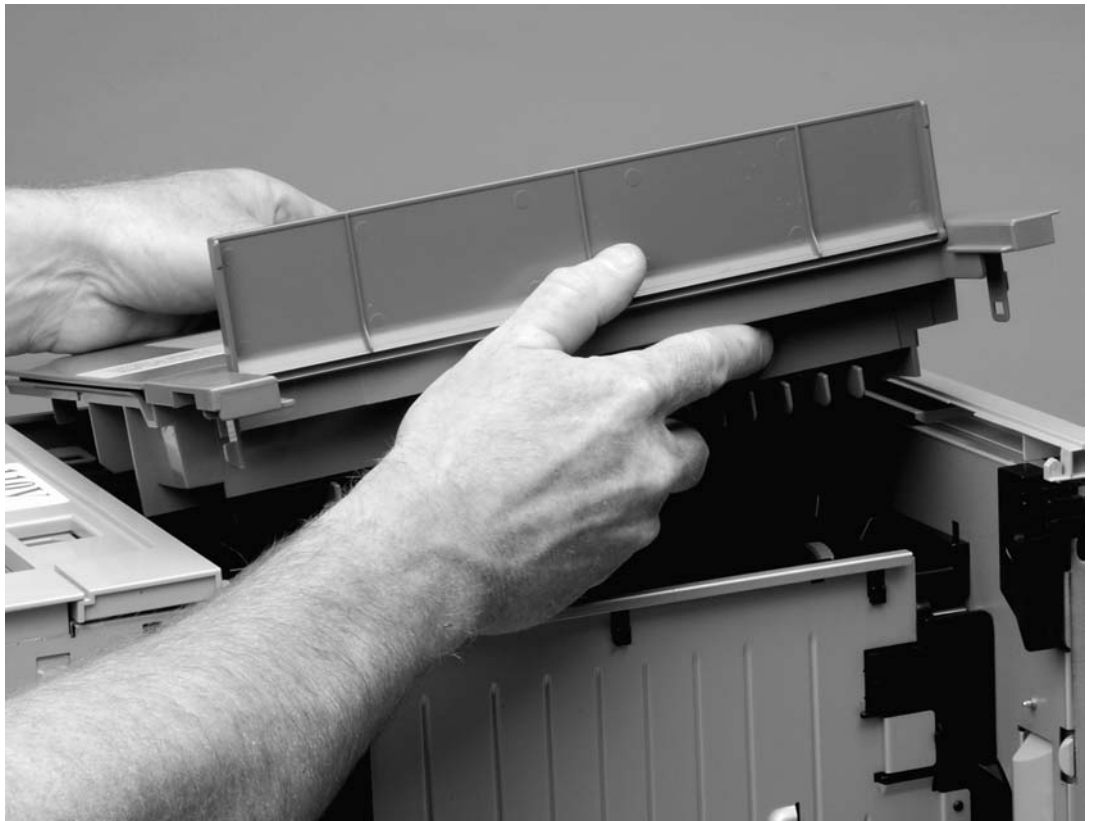
Figure 6-5. Removing the back cover (3 of 3)
