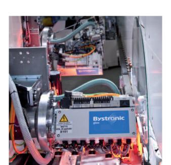
flexspacer'twinapplicator with two alternately functioning application heads
