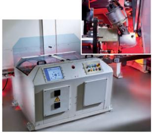
cornersealer for secure corner sealing via tape adhesion and an additional butyl sealing (optional)
