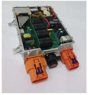
The 6.7kW OBC using VisIC GaN power devices targets plug-in hybrid vehicles/electric vehicles (PHEV/EV) applications. With a universal 110-220V/16-32A AC input and 200-430V DC output for charging the automotive battery by controlling voltage and current flow to the battery. The charger is designed to provide the interfaces to charging standards on the input power side and thus adapts to charging infrastructure.
