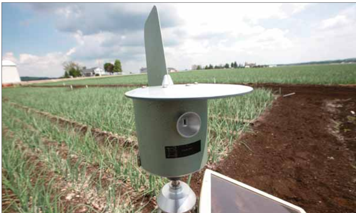
This trap collects spores in a vial each day. Stemphylium leaf blight, for example, can be identified by its spores using molecular means. Twenty years ago, this modern spore trap was not in existence nor was the disease found in onions in the Holland Marsh north of Toronto, Ontario.
