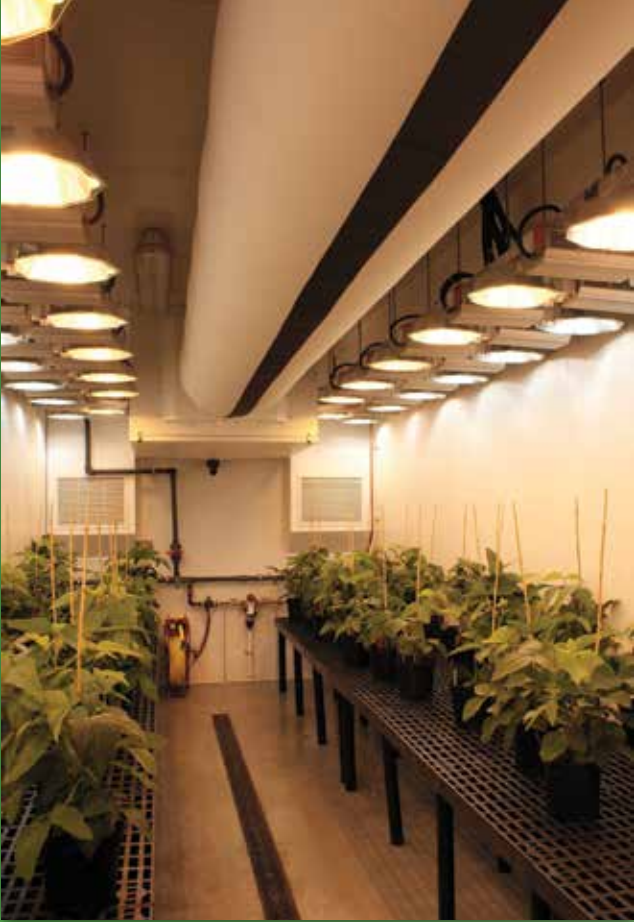
Stability Chamber: Vertical draft in center creates uplift through plants to return air.
