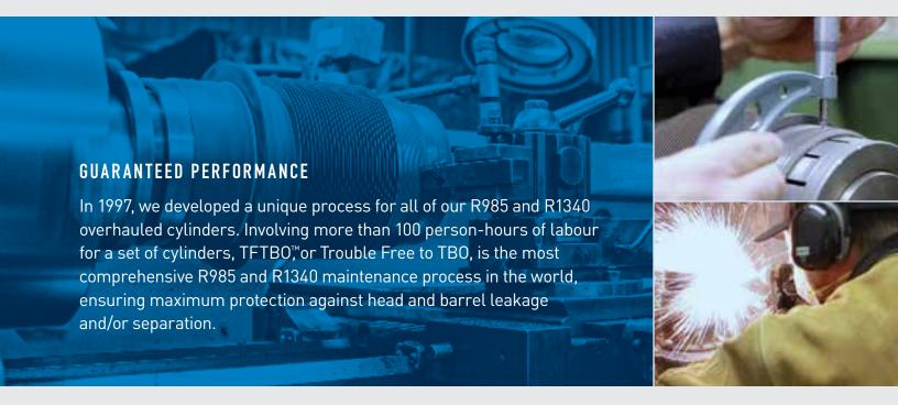
Cylinders are given new life by paying close attention to the thread and barrel interface and the interference fit between them. A rigid visual, liquid penetrant and ultrasonic inspection for cracks enables us to identify the cylinders at risk of having head and barrel leakage or separation issues.
