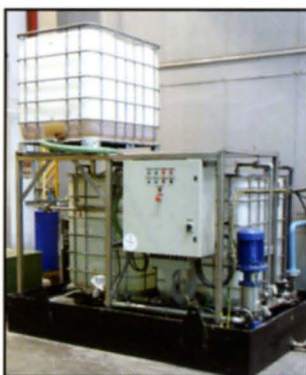
Preparation skid for on-line and off-line washing for a 280 MW gas turbine.
