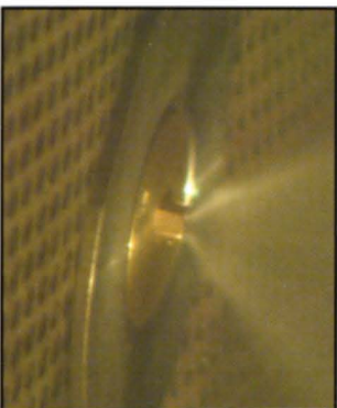
The Mk 3 air-assisted nozzle in action on a GE Frame 9E operating at base load.
