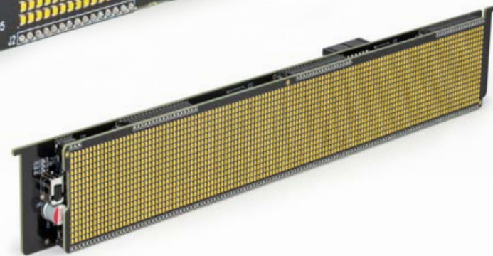
The Select DAC display is huge and comprises 2096 individual LEDs
