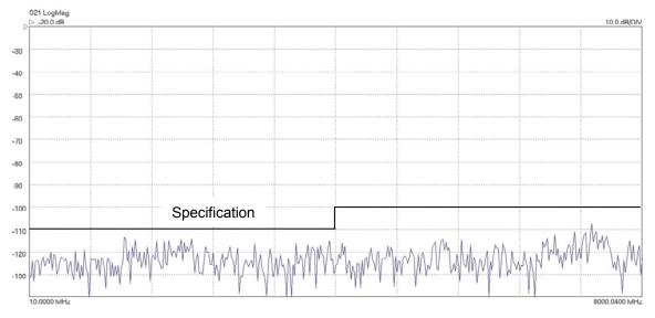
Measured wideband (10MHz to 8GHz) system dynamic range excluding crosstalk (P<sub>test</sub> = +6dBm, BW=20Hz and 16 averages)
