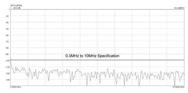
Measured low frequency (0.3MHz to 10MHz) system dynamic range excluding crosstalk ( $P_{test}$  = +6dBm, BW=20Hz and 16 averages)
