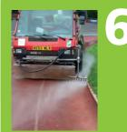
The edges of athletics tracks can be cleaned using a side arm.
