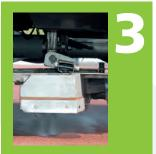
The cleaning phase begins with low pressure, high volume water jets being used. These don't damage the surface or line markings.
