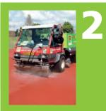
Using our unique Aquatrax® machine, the first pass is the 'pre-wet' phase – holding the dirt in suspension.
