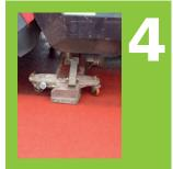
A vacuum, integral to the Aquatrax® machine, then removes the dirty and contains it until disposal.
