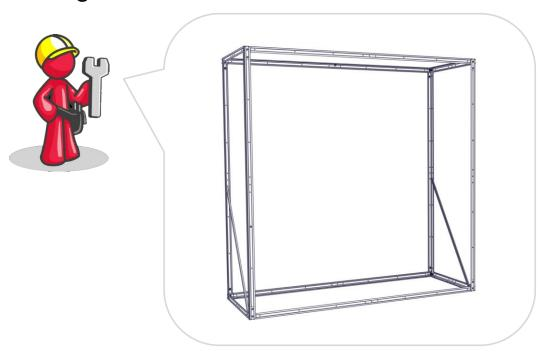
Step 3 - Bolt together the two end assemblies using horizontal sections
