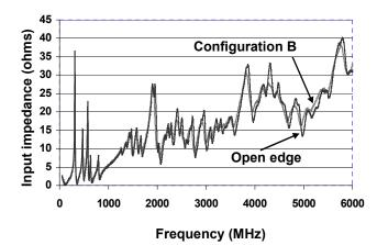
Figure 10. Comparison of input impedance of open edge board with that of board with absorber mounted as in "configuration B" as defined in figure 8. There are only small differences in impedance between these cases.
