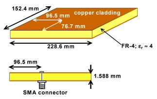
Figure 2. Experimental structure without absorber (not to scale).
