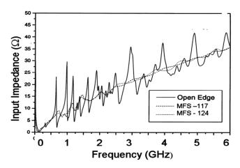
Figure 7. Theoretically calculated input impedance as function of frequency for the three configurations whose measurements are displayed in Figures 5 and 6.
