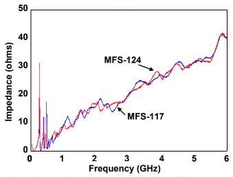
Figure 6. Input impedance as a function of frequency for two circuits with MFS-117 and MS-124 absorbers on their perimeter.
