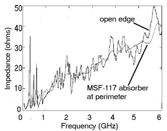
Figure 5. Input impedance as a function of frequency for an open edge circuit board a circuit board with an MFS-117 absorber on its perimeter
