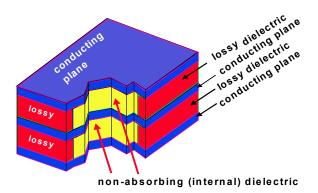
Figure 1. Basic structure of perimeter-absorber board.
