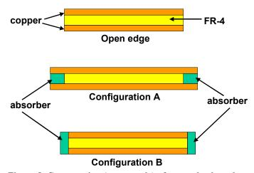
Figure 8. Cross section (not to scale) of open edge board and two methods of mounting the absorbing material.
