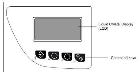
The function of the command keys differ according to operating mode of the equipment.
