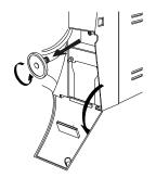
When it is due to be changed, or when you notice visible clogging of the filter (indicated by a color markedly tending towards gray) unscrew the bacteriological filter from its support and replace it with a new one by screwing it all the way down on the connector on the front of the machine.
