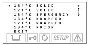
Using the + and - keys, scroll the list until you identify the sterilization program desired.
