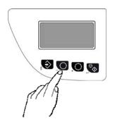
To select the **VACUUM TEST** program, press the **Test Selection** key one or two times until the display reads:
