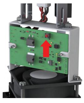
If the unit was manufactured before Nov. 2016, The red reset button will be located on the vertical circuit board.
