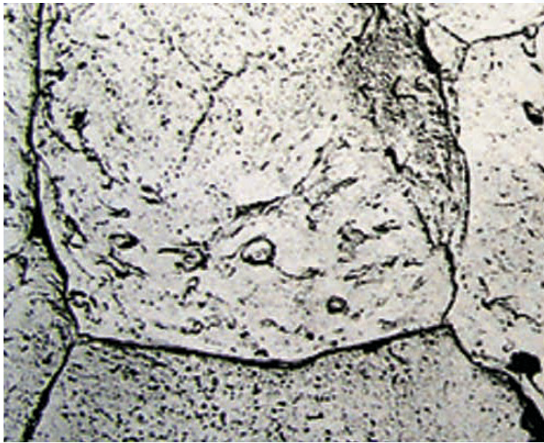
An electron micrograph of a “clean” silver soldered joint. Note the crack lines and other impurities of the melted metal.
