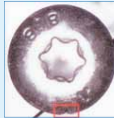
Kopfriss Head Crack
