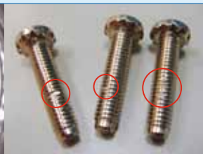
360° Degree Thread Damage Inspection (Customized)
