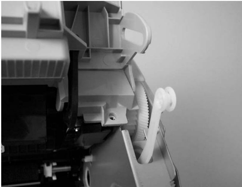
Figure 5-11 Remove the rear panel and top-cover assembly (3 of 6)
