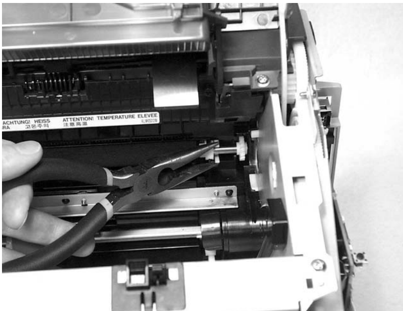
Figure 5-22 Remove the transfer roller (3 of 3)
