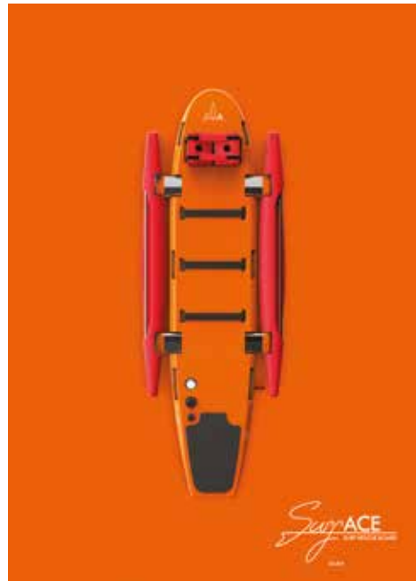
ARCHIE ASHFORD MEng Product Design and Manufacture Surface is the first surf rescue board designed to aid lifesavers in the treatment of neck and spinal injuries. Using water as ballast, Surface can be submerged and re-surfaced to safely transfer patients onto the board.
