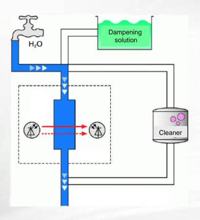
ALCOPRINT = automatic zero-point synchronization by periodic rinsing of the measuring chamber with IPA-free industrial water.
