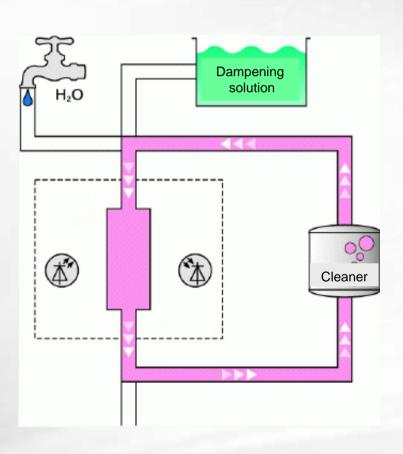
If required, a cleansing cycle is initiated automatically using a detergent in a closed circuit
