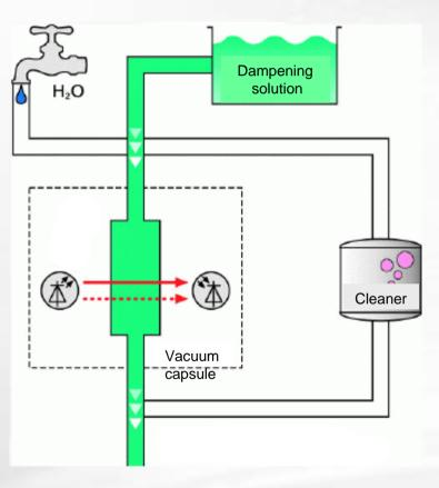
ALCOPRINT selectively measures the level of isopropyl alcohol. Measured values are therefore not influenced by other components of the dampening solution.
