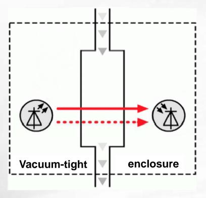
This eliminates the risk of optical and sensor component contaminations and any measuring errors they may cause.
