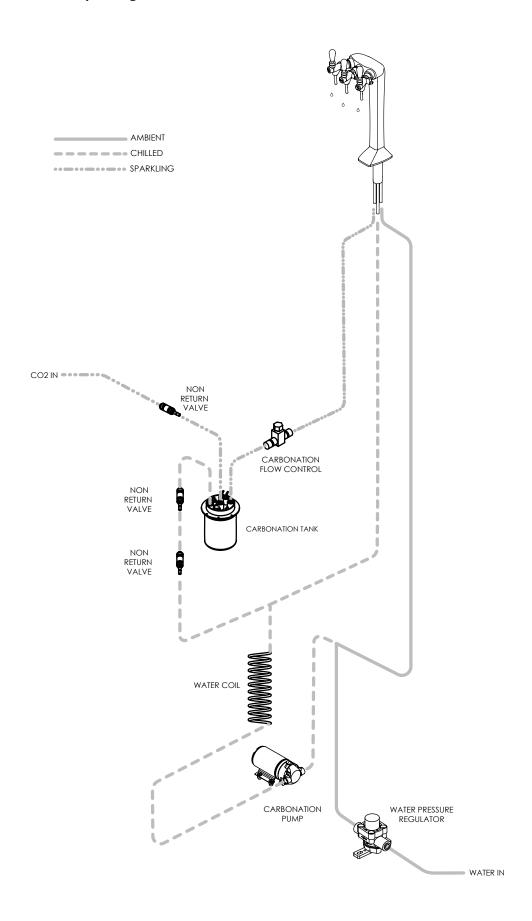
Chilled & Ambient Water Pathway Diagram - Water Pathway Diagram
