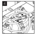
Flow can then be adjusted by turning the adjuster screw, anti-clockwise to increase flow and clockwise to restrict flow. After each adjustment the flow rate should be timed.
