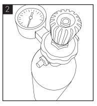
Attach the regulator to the disposable CO2 bottle, ensuring the small pressure relief vent in the stem is facing away from you or anyone else. Ensure the regulator is closed. Hand tighten securely.
