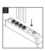
Connect the u2 tap to the Chilled, Ambient and Sparkling\* water outlets.
