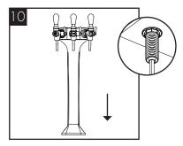
With the tap in position carefully refit the nut. Take care not to over-tighten.
