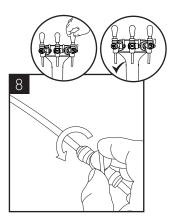
\*Isolate the water supply and activate the sparkling water dispense. When the water system has emptied, allow gas to be expelled for approximately 5 seconds. Immediately after this 5 second period restore the water supply and allow the system to refill.
