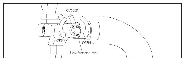
Use the valves on the sides of the taps to increase or decrease flow rate. Lever in the upright position is fully closed.
