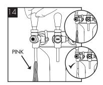
When the external cleaning (minimum 5 minutes) is completed, flush the machine using the cold dispense lever with clean water until the dispense water runs clear. Repeat briefly with the ambient and sparkling levers if present.
