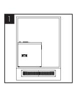
Locate the machine in a suitable enclosure, ensuring that the supplied ventilation kit can be installed.
