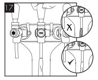
Pre-flush the new filter to waste using the ambient dispense lever until the water appears clear and is free of air. Flush through a small amount of water to check all functions.
