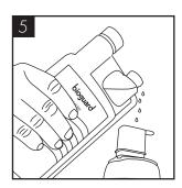
Add 25 ml of Bioguard Internal Sanitisation fluid to a clean and empty service filter cartridge.
