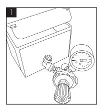
Unpack CO2 Regulator and fit elbow fitting to spigot outlet.
