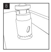
Carefully form the needed hole, using the correct type of cutter for the work surface material.
