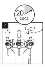
\*The carbonator should be purged of air by activating the sparkling water dispense for approximately 20 seconds.
