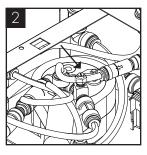
Locate the flow control adjuster, this can be found on top of the carbonator can, connected to the central port of the can.
