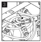
Loosen the lock nut, but do not remove.
