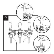
Dispense ambient, still and sparkling water\*, in turn, to purge any air from the system. The time to do this may vary depending on the length of pipe between the unit and the tap.
