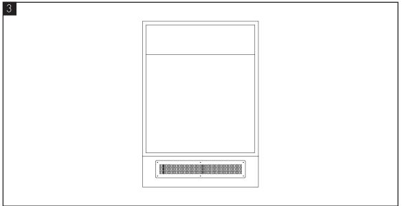
Centrally locate the ventilation grille over the kick board cut out, then using self tapping screws, secure the kick plate.
