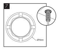
Allow sufficient space for fitting a back nut to the faucet stem.
