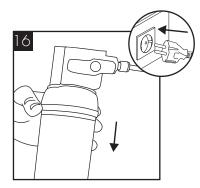
Fit new filter. Turn on incoming water supply and reconnect the power.
