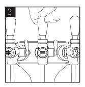
Briefly dispense cold/ambient water to release internal water pressure from the machine.
