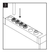
Connect the assembled CO2 bottle and regulator to the CO2 inlet using a 1/4 " pipe.
