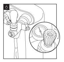
It is necessary to prime the sparkling system with CO2 - using the sparkling dispense lever for a few seconds until CO2 is coming through, check and adjust the CO2 pressure accordingly
