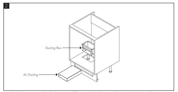
Insert ducting box into its cut slot in the Bottom panel. Then insert the air ducting into the ducting box until it reaches its limits. Then cut the air ducting so that it is flush with the kickboard.
