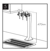
Also allow for the height of the tap levers under any overhanging cupboard/shelf.
