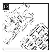
Remember to include the drip tray. If a Waste Overflow System is fitted, empty this and flush through with a small amount of sanitisation fluid if needed.
