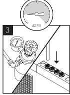
\*Connect the CO2 supply from gas regulator, ensuring the pressure is set to 58 PSI (4 bar), and turn on the supply.
