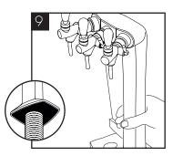
Remove the back nut from the tap and carefully feed the connecting pipe tails through the hole formed in the work surface. Ensure the rubber gasket is positioned correctly on the base of the tap.
