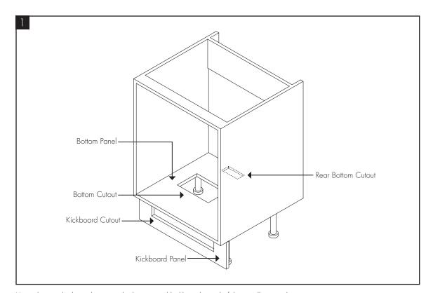
Using the supplied templates, cut the bottom and kickboard panel of the installation cabinet.
