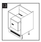
Once the ventilation system is installed, position the unit on the ducting as instructed and follow the connection steps on page 9.
