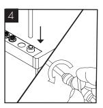
Connect the chiller to the water supply and open the mains supply isolation valve.
