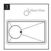
Identify a suitable position for the tap. A 50mm (max) hole is required for a three headed tap, and a 35mm (max) hole for a two headed tap.
