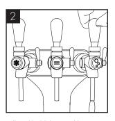
Pull and hold the Sparkling water dispense lever until all the water is expelled and only CO2 gas is being released.
