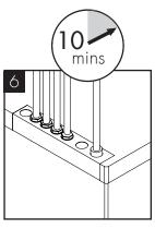
After approximately 10 minutes, the compressor and fan will stop as the chiller has reached its normal operating temperature.
