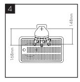
When positioning to drain over an existing sink bowl, allow for the reach of the tap levers or otherwise the position of any optional drip tray. 168mm to middle tap, 148mm to outside taps.
