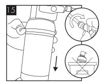
Turn off water and remove the service filter. Retain service filter for reuse.
