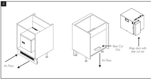
The unit must be positioned accurately over the air ducts to ensure optimum airflow.
