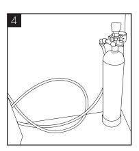
Stand the cylinder in a suitable place.
