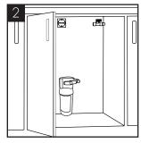
When planning and providing for the connection to the services, always allow for easily accessible service isolator fittings and for the position of an external water filter.
