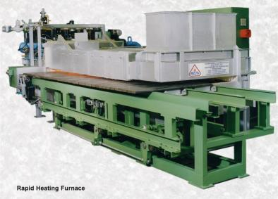
Gas Fired Rapid End Heating Furnace with Walking Beam and Roller Conveyor discharge designed specifically for the end heating of plates prior to parabolic rolling for commercial vehicle leaf springs.
