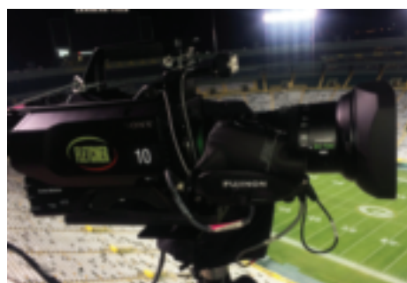
Fujinon PL20-120mm Cabrio lenses, in conjunction with Sony's HDC 4800 cameras, is helping ESPN shoot goal-line close-ups of the Monday Night Football programme.
