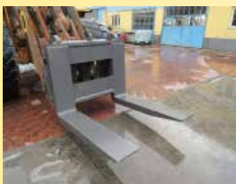
Forks for stone blocks for Loader Volvo L220 - forks capacity 48 tons
