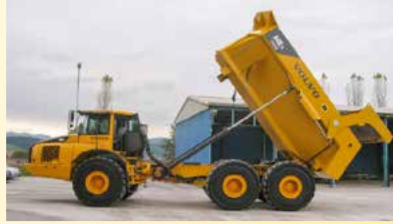
Volvo A40E with body for light materials made on Balavto Ltd.
