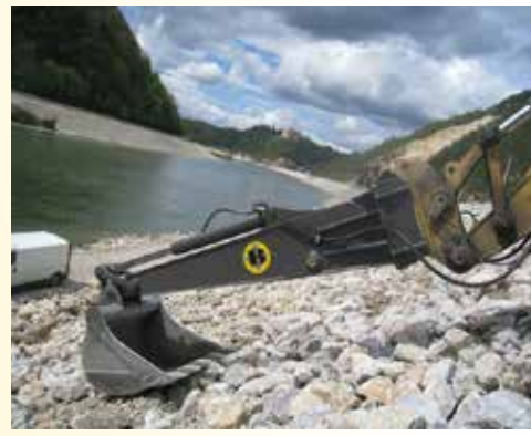
Underwater digging - Arm extension enables digging in positions that are much below excavator level - for example digging in the water (sea, river ...)
