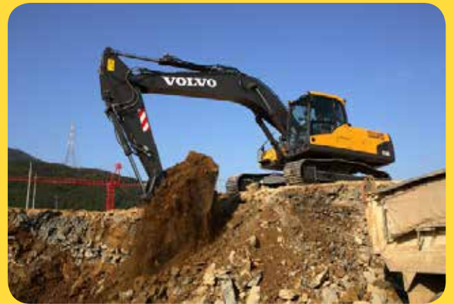
Volvo EC240 with Standard 2,5m arm - digging reach 9,8 m
