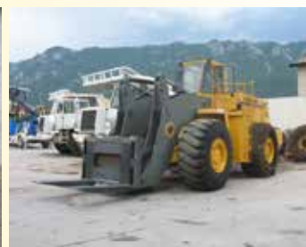
Forks for stone blocks for Loader Michigan L270 - forks capacity 60 tons
