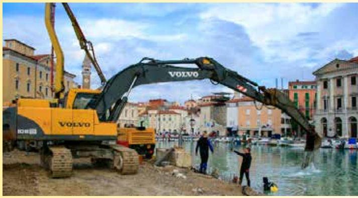
Underwater digging - Arm extension enables digging in positions that are much below excavator level - for example digging in the water (sea, river ...)
