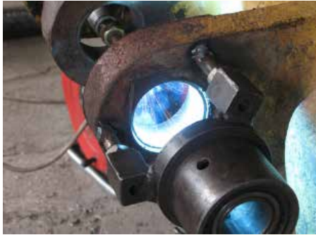
Repairing the old and demaged pins and bushing
