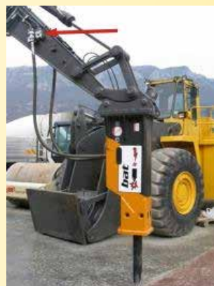
Hydraulic Breaker and Hydraulic Shear, both connected to excavator with B-Quick coupler
