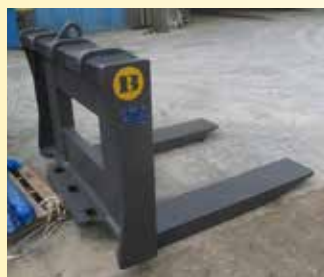
Forks for stone blocks for Loader Michigan L270 - forks capacity 60 tons
