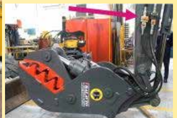
Hydraulic Breaker and Hydraulic Shear, both connected to excavator with B-Quick coupler
