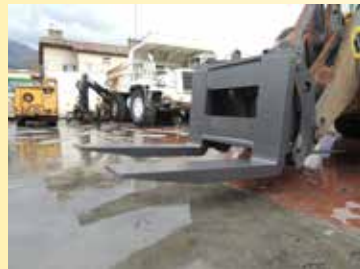
Forks for stone blocks for Loader Volvo L220 - forks capacity 48 tons
