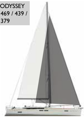
Large overlapping genoa Performance / Génôis Performance à fort recouvrement / Genua in starker Überlappung Performance / Génova con mucho recubrimiento Performance / Genoa a forte recupero Performance
