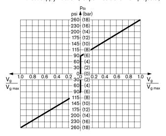
$V_g$  displacement at  $p_{St}$   $V_{g max}$  displacement at  $p_{St}$  = 260 psi (18 bar)
