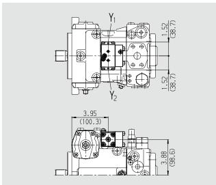
Electric two-point control with switching solenoid, EZ
