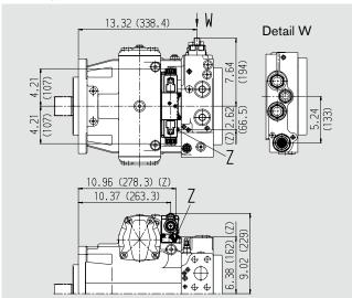
Control valve, fixed setting and ports for pilot control device, DA7
