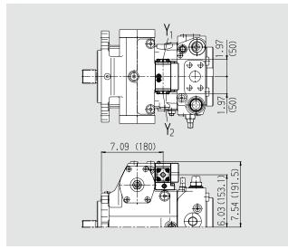
Electric two-point control with switching solenoid, EZ
