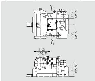
Electric two-point control with switching solenoid, EZ
