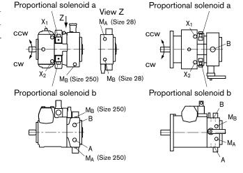
Standard: proportional solenoid without manual emergency operation. On request: manual emergency operation with spring reset available.
