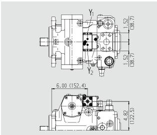
Electric two-point control with switching solenoid, EZ
