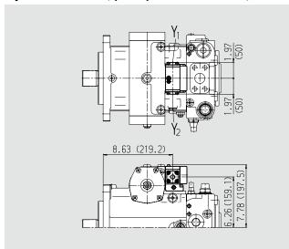
Electric two-point control with switching solenoid, EZ
