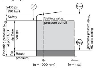
Note: valve is set at n = 1000 rpm and  $V_{g \text{ max}} (q_{v 1})$
