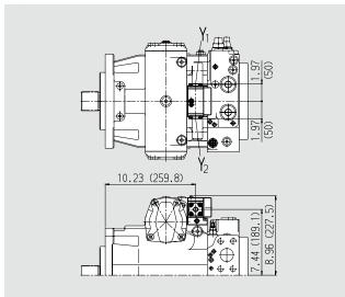
Electric two-point control with switching solenoid, EZ
