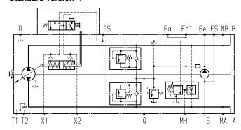
Version with DA control valve and neutral position switch 1)
