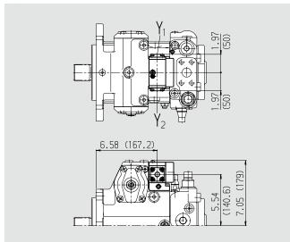
Electric two-point control with switching solenoid, EZ
