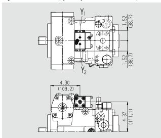
Electric two-point control with switching solenoid, EZ
