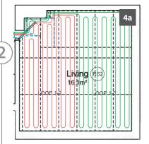
Before attempting to lay any floor heating boards, familiarise yourself with the system layout drawing, noting manifold position. The drawing will detail the orientation and position of panels (4a).
