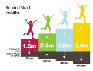
MonsterPlay@Caloo Bonded Mulch has been tested to the strict requirements of BS EN 1177:2008 on a concrete base in laboratory conditions (worst case scenario).
