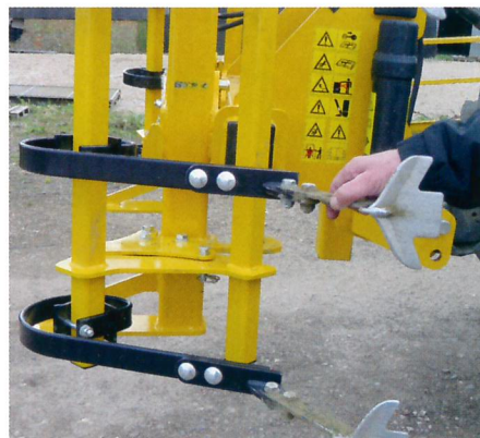
The TerraBlade's flexible leg allows the share to ride over the surface at up to 7km/hr.
