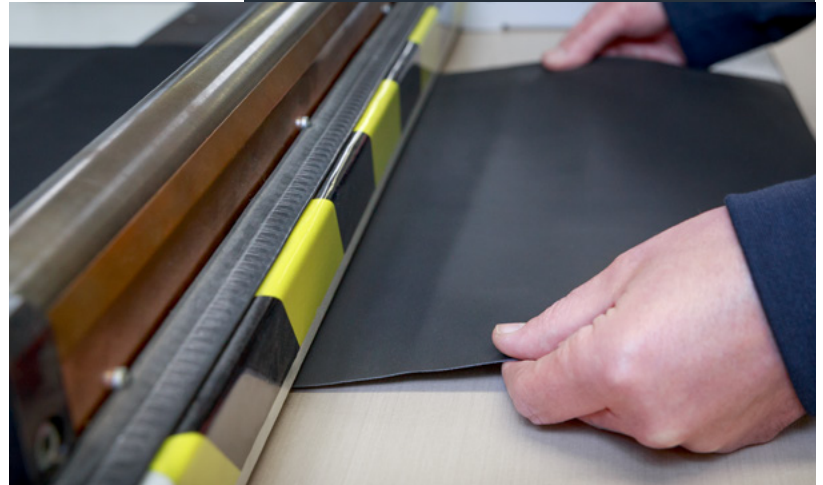
Splitting: Leather being split to a uniform thickness
