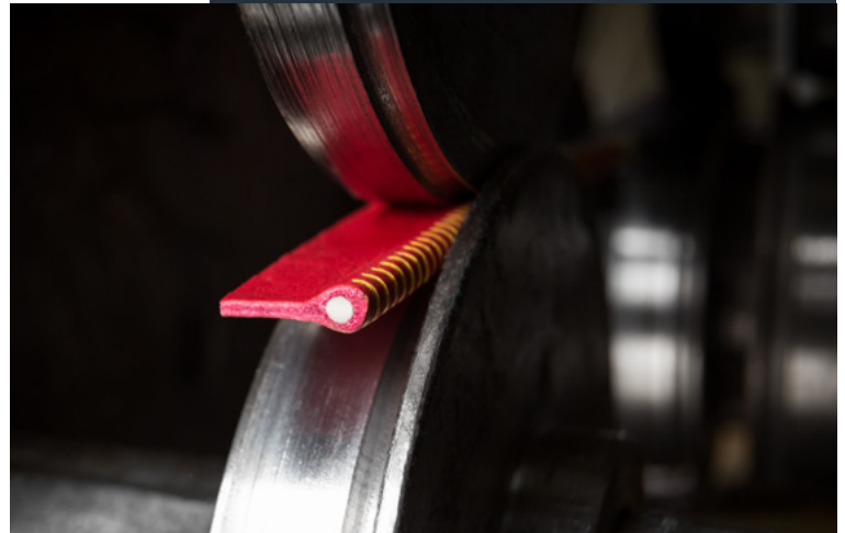
Piping machine: Example of piping with a solid core.
