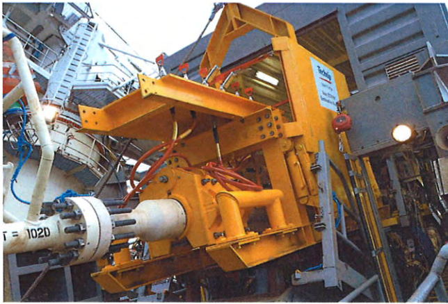
Figure 6. Islay ETH termination assembly on Apache II .
