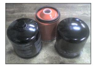
Air dryer cartridges are the best possible protection for pneumatic braking systems. In the field of safety, brakes are amongst the most important components of a vehicle and dry, clean air is particularly important for the pneumatic braking systems on trucks and buses in order to protect the system from corrosion and malfunctions. Our range of air dryer filters solves this problem.
