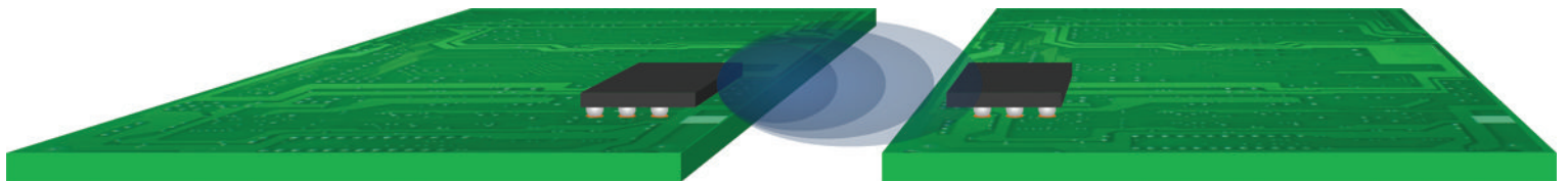
The WaveConnex product concept uses 60GHz EHF energy to transmit Gbps signals across short-reach gaps between printed circuit boards.
