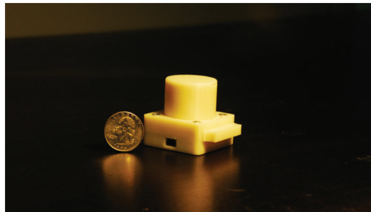
Prototype for Ozcan's lensless microscope.
