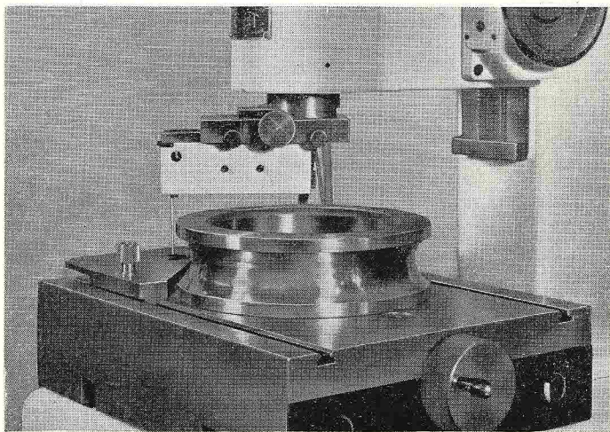
12 Close up view of a set-up on an O.M.T. roundness measuring machine, fitted with a Foxboro recording instrument, which is installed in the central metrology department of the Peterborough works. This set-up provides for checking the dimensional accuracy and roundness of the track in a ball bearing inner race. Another set-up on the same machine serves for checking the circularity of cross-section of the track, and for this purpose the inner race is supported in a vice type fixture with its side faces vertical
