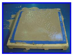
Aggressive vibration can lead to segregation and also cause spillage of concrete out of the mould.
