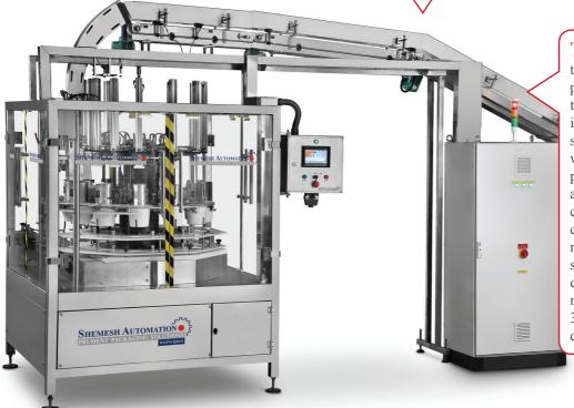
The SAS120 is offered in throughputs of 60, 120 or 200 products per minute. It feeds the round wipes vertically into a 90° chute to the main servo-driven rotary turret where a pneumatic piston pusher stuff each roll accurately into its designated canister. Saving downtime, it is designed for ultra low sub 30 minutes changeover and can stuff canisters with rolls that don't have to be tighter, but may actually be wider by up to 3mm than the canister outside diameter, a big plus.
