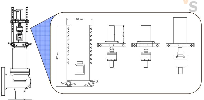
The rig consist of the metal bars and three bridges (1 kN •10 kN • 20 kN). A bridge includes a hydraulic cylinder and a force sensor.
