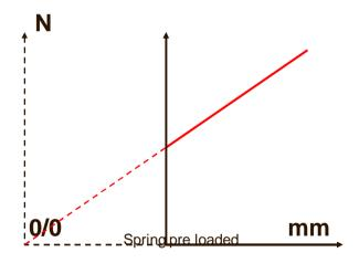
$F_{Spring}[N] = C[N/mm] \times \Delta X[mm]$
